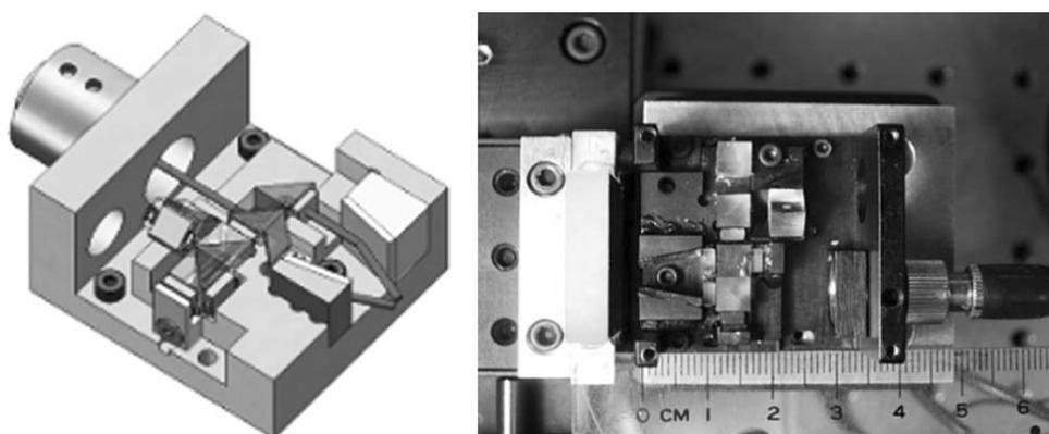
**Figure 6** (a) The structure of the LDGI; (b) The photo of the LDGI.
