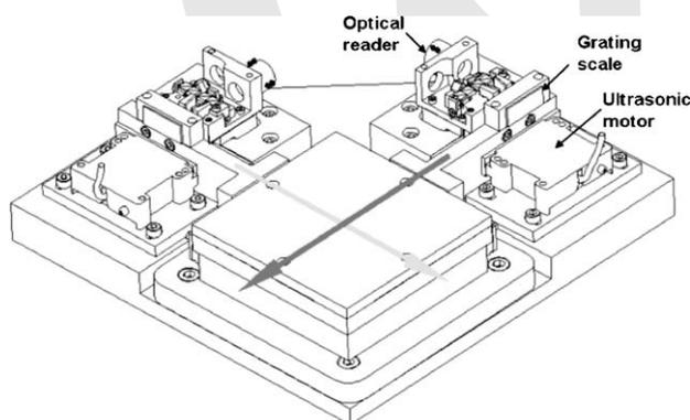
Figure 2 A co-planar stage of push-pull driven type.
