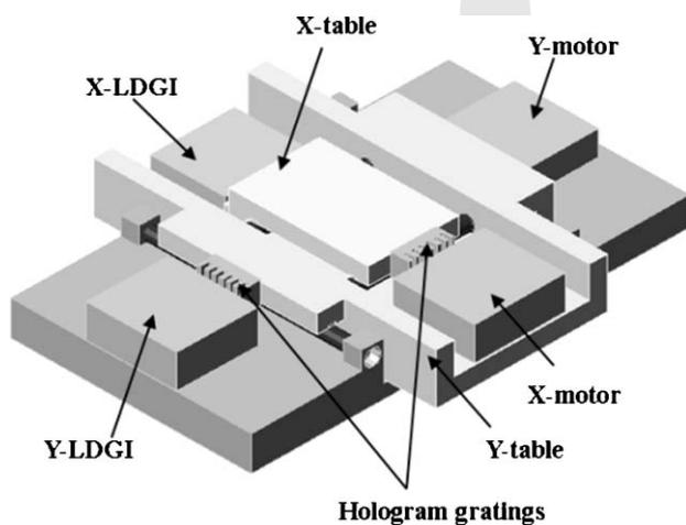
Figure 1 A co-planar stage of side-driven type.
