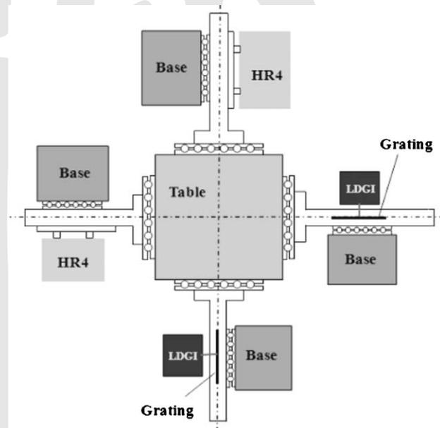
Figure 3 The symmetrical push-pull co-planar stage.
