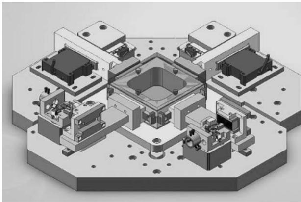
Figure 4 Structure of the co-planar stage.
