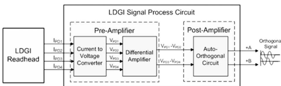
**Figure 7** The circuit diagram of LDGI signal process.
