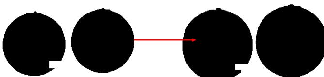
Dilate 3 times (**radially**) to diminish the influences of the defect on the averaged coordinate of the sphere (more black/less white pixels).
