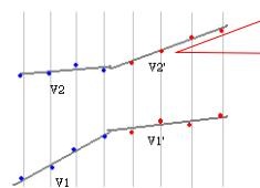
We can fit a line through 4 position data points and use the slope for the sphere velocity.
