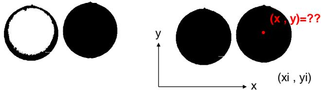
Due to the greater number of 'solid' pixels, the estimated sphere center is less sensitive to the BW image manipulations.
