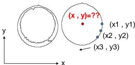
Large deviation due to the thin line that defines the edge of the sphere
