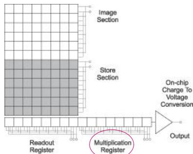
EMCCDS use similar structures to CCD's, but prior to being readout at the output node the charge is shifted through an additional register—the multiplication register—in which the charge is amplified.
